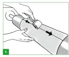
Particular care is required when pushing the ORAFLEX® tape into contact with the plate edges to avoid edge lifting especially on the leading and trailing edge.
