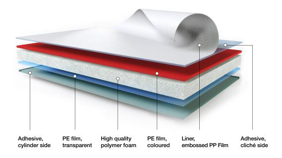
The **ORAFLEX®** Cushion Tapes' compressible foam and film reinforcement construction technology guarantees an optimized thickness accuracy, with minimal thickness tolerances (+/- 0.02 mm).
