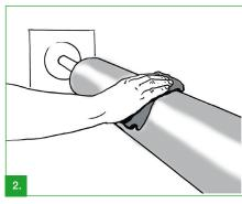
Clean the print cylinder per manufacturer recommendations and wipe dry with clean lint-free cloth. Make sure it is completely free from dust and other contaminations (e.g. ink or adhesive residues). Recommended solvent to use is isopropyl alcohol. Solvents like ethyl acetate should be avoided and can strongly affect adhesive performance. Ensure the surface is totally dried before mounting.
