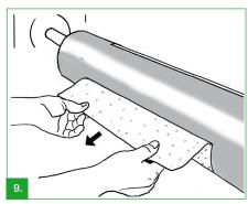
Pull back the ORAFLEX® cushion tape from the cylinder and remove it. The printing cylinder / sleeve and plate should be cleaned before the next use.
