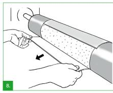
For demounting: remove plate first. To avoid stretching of the plate the peel angle should be flat. Loosen the edges of the print plate and pull it downwards, detaching it from the adhesive side of the ORAFLEX® tape.
