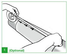
ORAFLEX® 11405 Edge Sealing tape can additionally be used to seal the plate edges on printing cylinders / sleeves with small diameter. Overlapping tape should be removed to avoid web breaks caused by contact of tape and print substrate.
