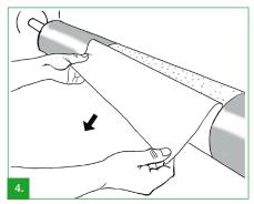
Pull down the liner and remove it from the ORAFLEX® tape without touching the adhesive.
