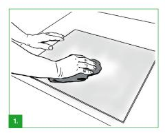
Clean the print plate. Make sure it is completely free from dust and other contaminations (e.g. ink or adhesive residues). Cleaning can happen with a suitable solvent and a lint-free cloth. Recommended solvent to use is isopropyl alcohol. Solvents like ethyl acetate should be avoided and can strongly affect adhesive performance. Ensure the surface is totally dried before mounting.
