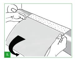
The print plate should be applied immediately after liner removal as dust might deactivate the open adhesive layer. Only fix the plate without pressure on a narrow area of the ORAFLEX® tape. Once the correct plate orientation is justified begin to apply the plate on the ORAFLEX® tape by using a rubber roller in a sweeping motion line by line.
