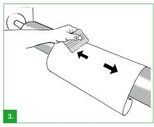
To avoid tensions in the adhesive bond the ORAFLEX® tape should be applied onto the printing cylinder / sleeve first. To avoid air entrapments apply the ORAFLEX® tape in a sweeping motion line by line on the printing cylinder. For best results use a squeegee or rubber roller.
