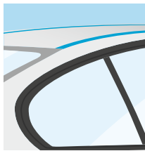
Roof ditch trim
